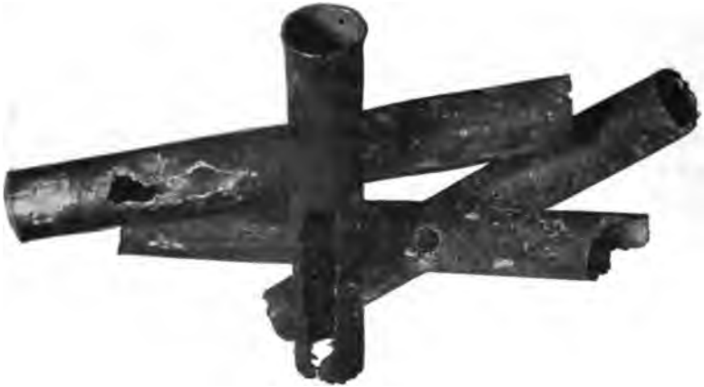
FIG. 24.—Effect of Electrolysis upon Brass Tubes
